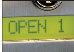
built-in display indicates door/gate has been opened
