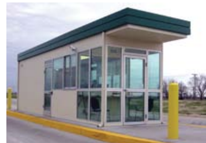
31'x8' Durasteel PC with integral visitors vestibule and 48" roof overhang, restroom, ducted heating and cooling system, custom painted stucco exterior finish, 16" high roof fascia with reveal and exterior floodlights.
